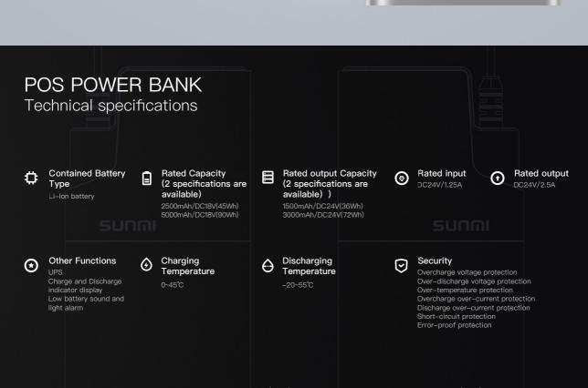
\*The POS power bank must be charged within the temperature range of 5°C~45°C and discharged within the temperature range of 0°C~45°C. If you charge or discharge the POS power bank beyond this temperature range, it will result in the drastic reduction of battery capacity and the shortening the use time.
